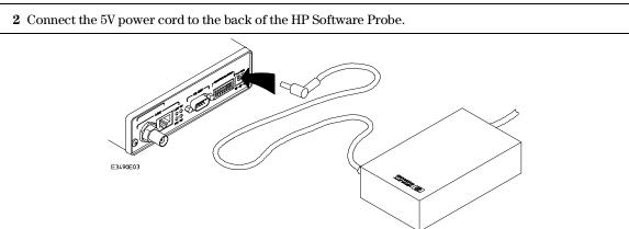
The power light on the target side of the HP Software Probe will be illuminated. The HP Software Probe does not have an On/Off switch.
